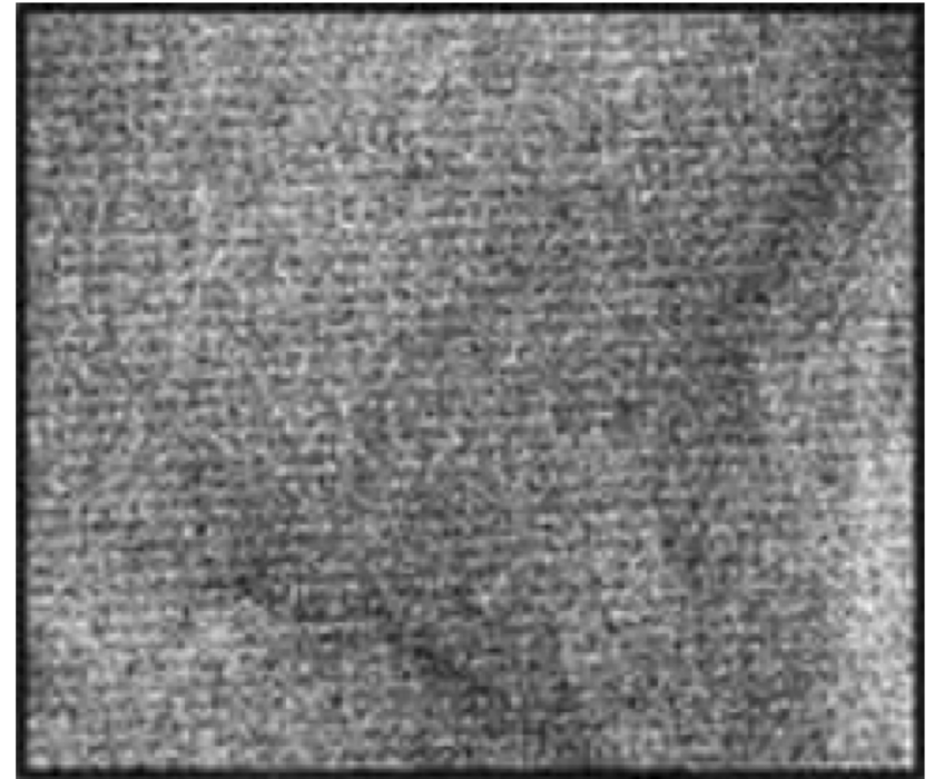
Scalloping on RADARSAT-1 ScanSAR Narrow A image
