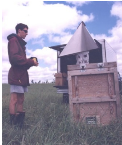
Corner Reflector (passive target)
